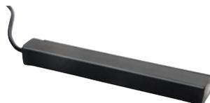
Larco's edge guards are manufactured to meet the user's specification for length. When pressed, the EGS110 and EGS120 edge guards send a signal to the safety controller to stop or reverse operation depending on the application. Multiple mounting channel designs allow for easy installation on most surfaces and provide a safety solution for narrow edges.
