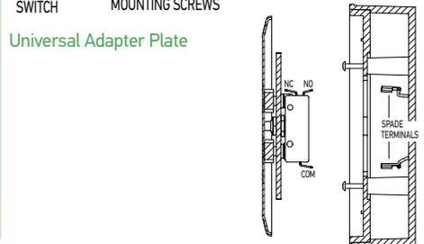
Push Plate Switch Wire Connection Drawing
