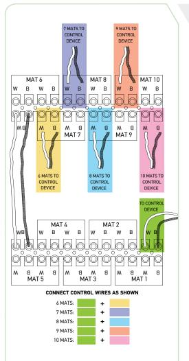
The black/white wires indicated above are from the supplied 4-conductor cable that runs from the junction box to the MAX Safety Relay or other safety rated control device.
