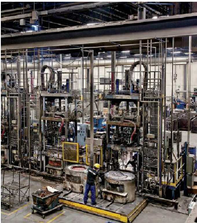
Atek Metal Technologies produces aluminum castings via the permanent mold process.
