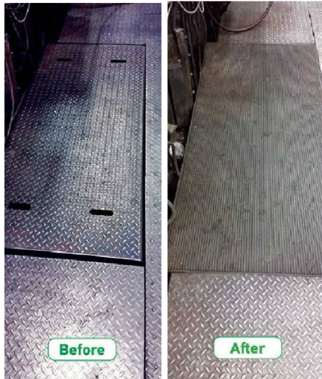
Atek Metal Technologies replaced steel pads utilizing spring triggers (left) with Larco safety mats designed to activate under 5 to 10 lbs. of pressure.
